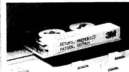
DC 100 Tape Drive Option 01 For workstation-type applications, the Option 01 built-in DC 100 tape drive provides convenient, menu-operated local storage and retrieval. It accepts tape cartridges (each holding up to 32 separate files) to store reference data, pattern generation programs, Extended Define Mnemonics tables or data acquisition setups.
